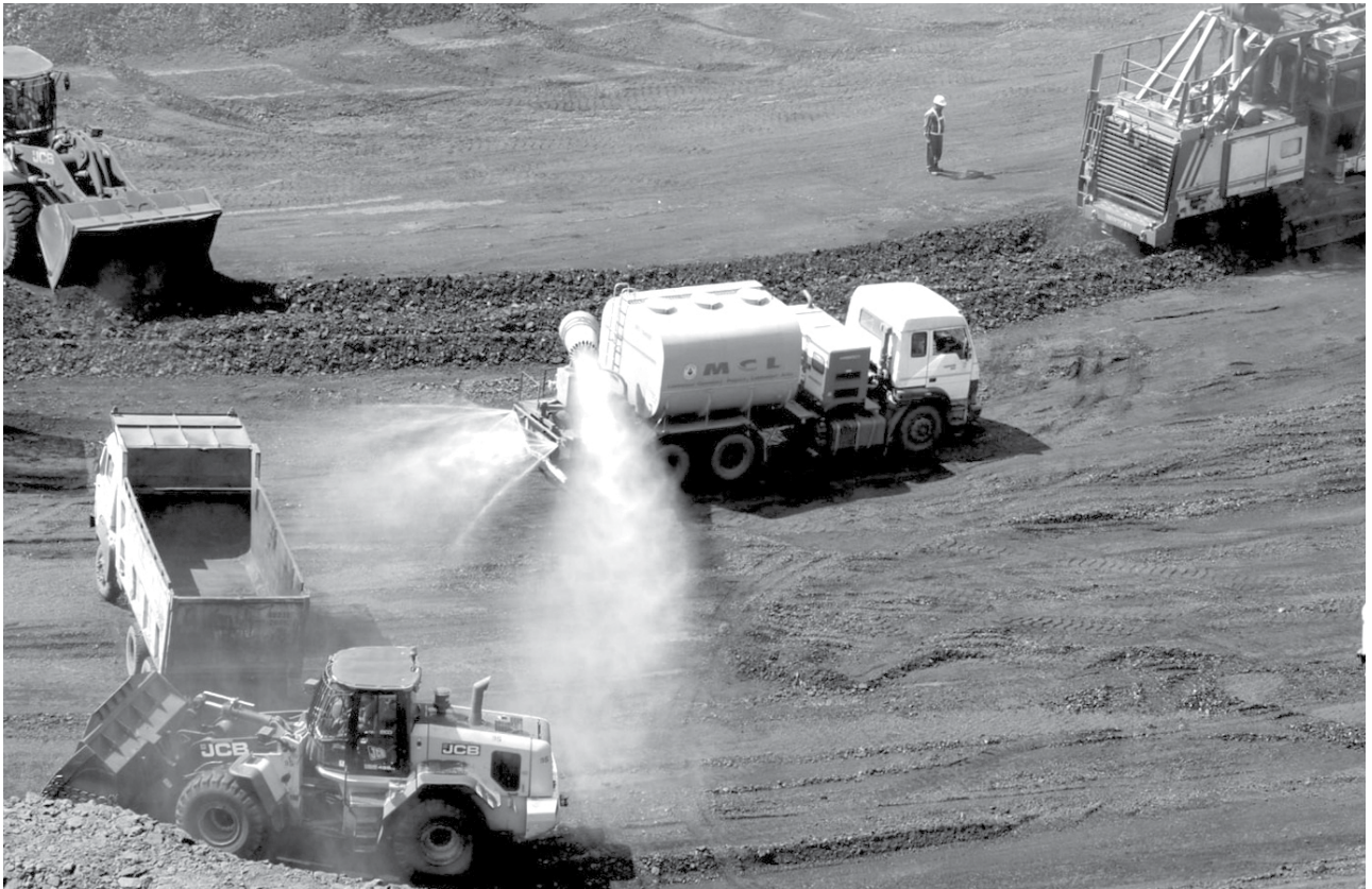
Effective dust control in surface miner face by fog cannon.
