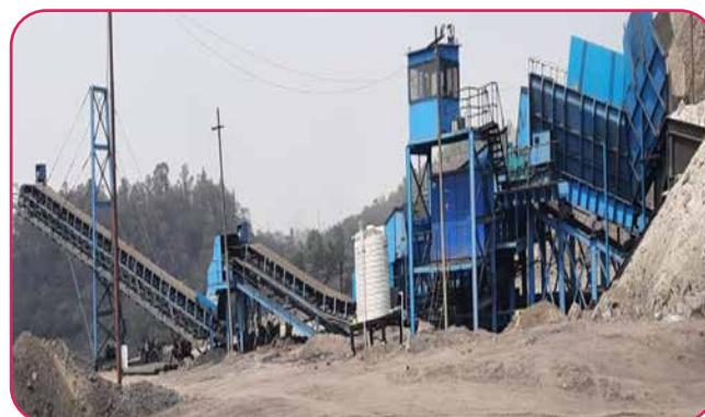
1000 TPH Mobile Crusher at Gevra Area
