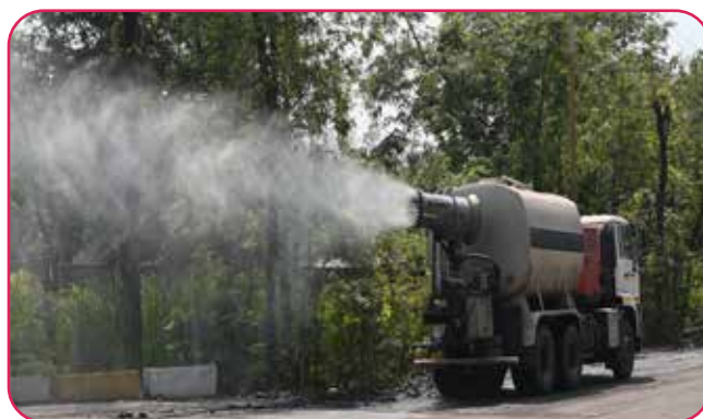
Truck mounted Fog Cannon Machine at Gevra Area
