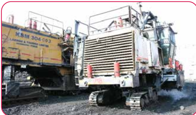
Surface Miner with inbuilt water spraying system
