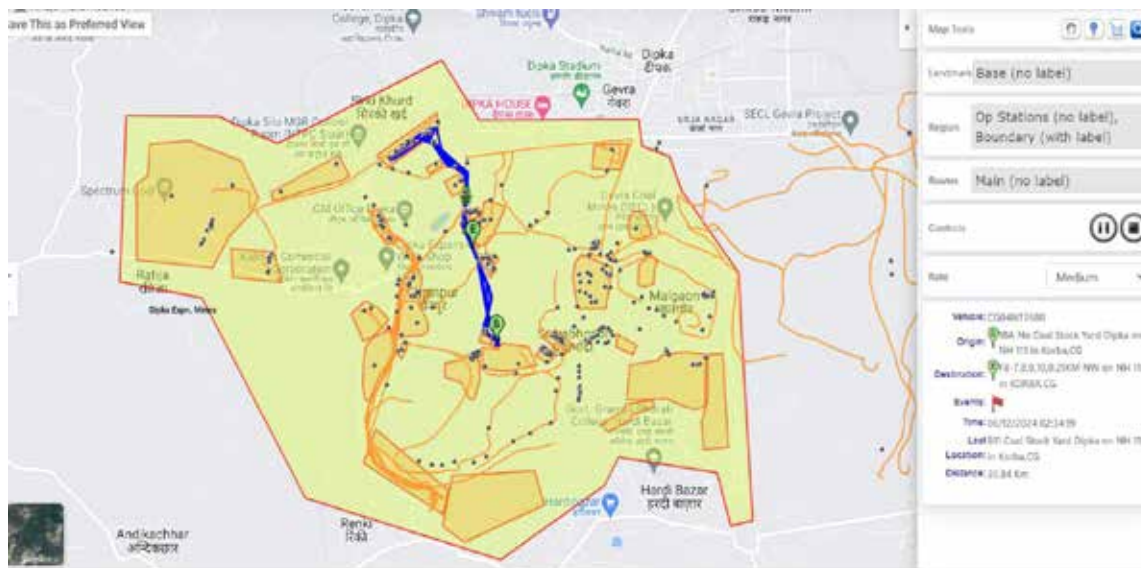
Geo-fencing of Mines, Siding & Authorized coal transportation route at Gevra Area (Blue line indicates Route Deviation)
