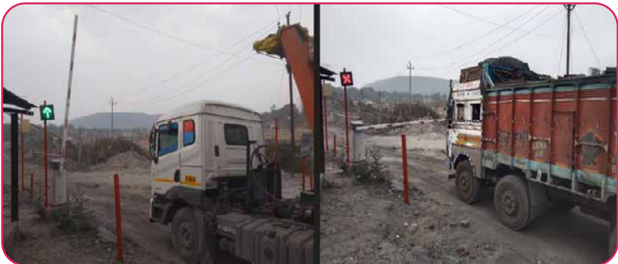
Barrier opens (Green light) for authorized vehicle
